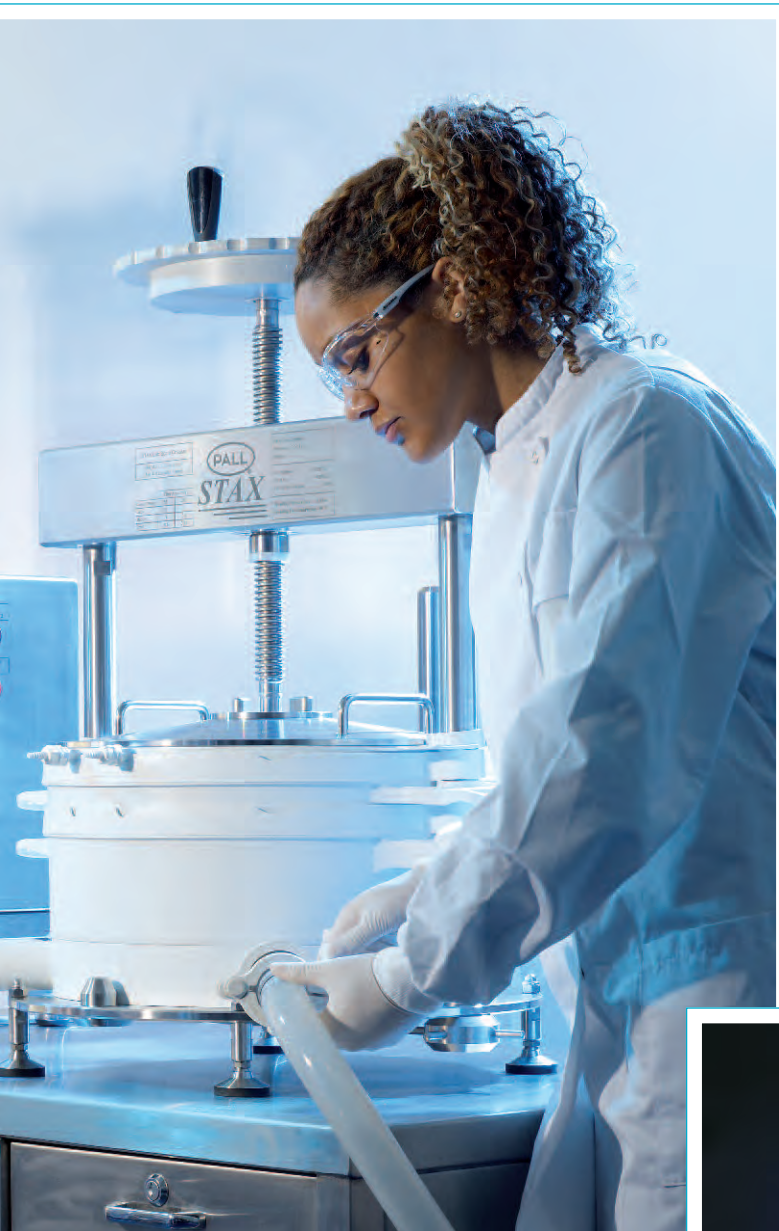
Top: Pilot Scale Chassis with Stax Capsules Right: Seitz Depth Filter Sheet Media
